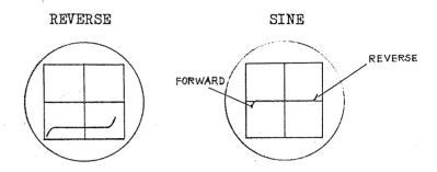
When tested under the SINE mode, if the sample is connected as indicated by the polarity indication mark on the test box cover, the polarity of the characteristics is as shown in the SINE pattern in the above illustration. If the sample is connected in the reverse, the polarity of the characteristics also is reversed.
